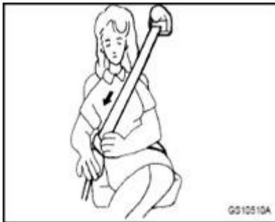
Pull the belt slightly to adjust looseness as desired.
